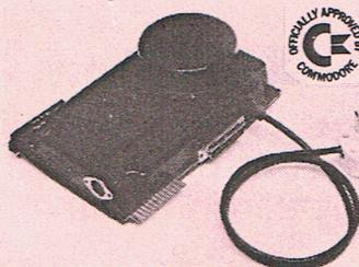
This fully implemented (true levels) bi-directional interface will allow the VIC 20 to operate as a Mainframe terminal, drive a Qume daisywheel, drive a paper tape punch, etc.
