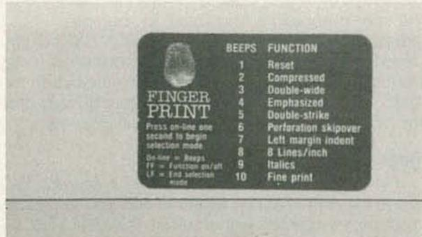
A LABEL AFFIXED TO THE FRONT of the printer tells what functions can be programmed directly from the printer's controls. This label for the IBM Graphics Printer shows 10 beeped functions.
